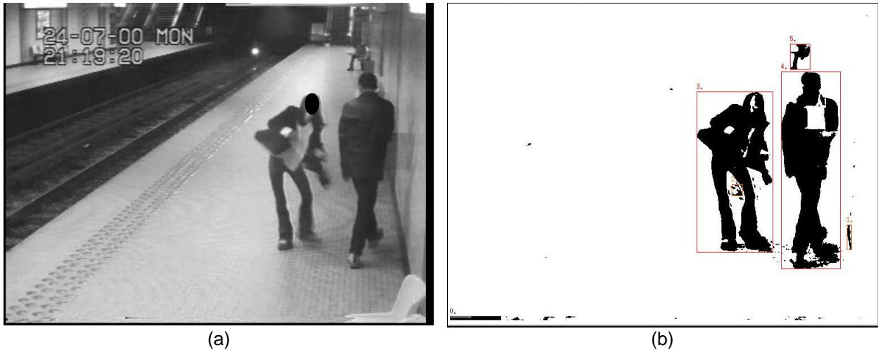
Figure 6: (a) raw image; (b) the moving regions represented by the red bounding boxes .
