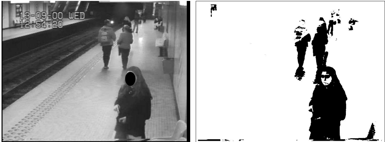
(a) (b) Figure 4: (a) raw image; (b) the black pixels are labelled "mobiles".
