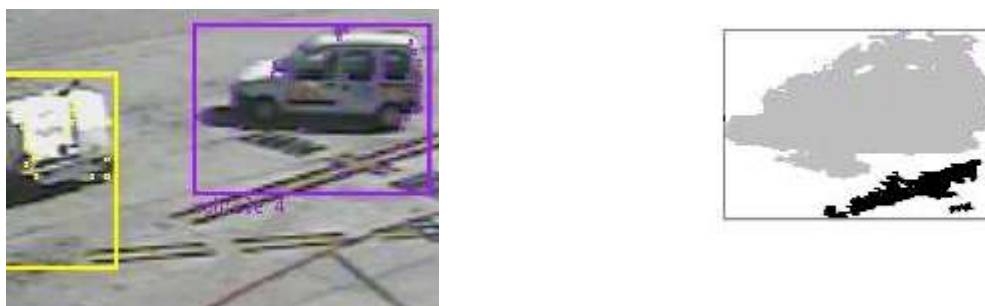
Figure 6: (Left) A van moving on the apron near paint markings. (Right) Reflections from the paint markings create spurious blobs (shown in black) in the motion detection results that are merged with the van's blob, creating an error in the van's 3D localisation.
