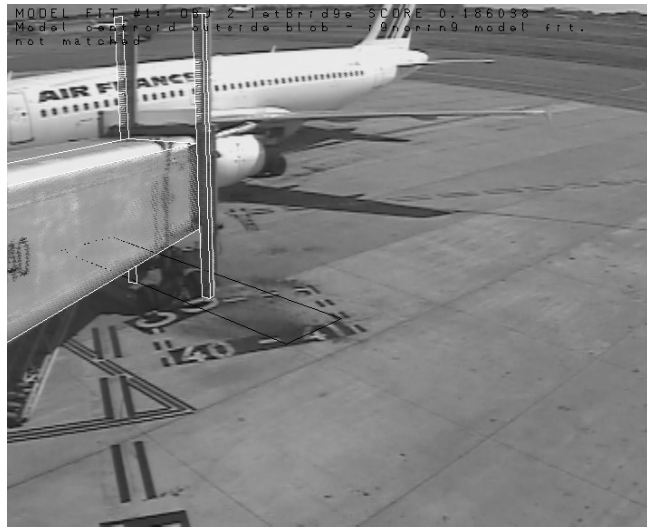
Figure 13: Using context-based search information (search region and orientation range) for specific objects. In this case the jet bridge can only be in a small set of positions. The X,Y search region on the ground plane is shown as a black rectangle on the apron.
