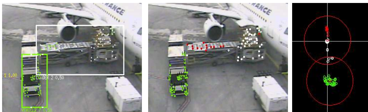
Figure 8: (Left) Sample frame from Dataset S28- A320 Camera 5 showing two vehicles (transporter on the left, loader on the right) that appear merged together for an extended period of time, while they move relative to each other. The transporter vehicle is moving slowly towards the camera, while the stationary loader vehicle is raising its platform. (Centre) Performing motion segmentation of the features of the 2 vehicles by fitting motion models and clustering. (Right) After performing clustering in the motion parameter space, 3 main motions are identified – a vertical motion displayed as red points that explains the upward motion of the loader's platform, a stationary motion (shown as white points) for the part of the loader vehicle that is stationary, and a forward motion (green) for the transporter vehicle.
