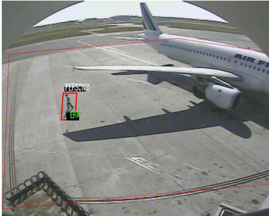
A person is inside the Equipment Restricted Area (ERA) zone
