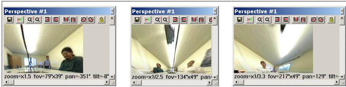
(e) Examples of views from cameras that are automatically tracking targets (with part of the omnidirectional image as backdrop). The program displays the fields-of-view of perspective cameras (colour-coded) in the omnidirectional image.
