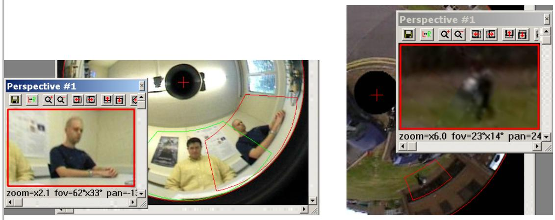
**Figure 6.15:** Different examples of perspective and panoramic views with camera control parameters applied to them
