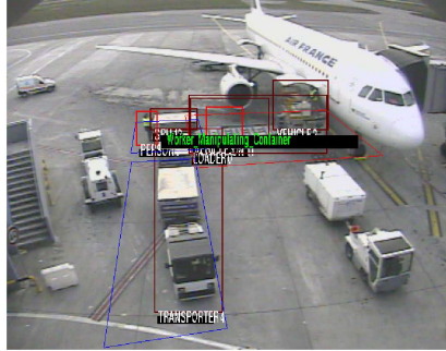
Fig. 3. (Left) Two dynamic zones (in blue) linked with the Loader and the Transporter vehicles involved in the event “Worker_Manipulating_Container” (event 26) detected. (Right) The Unloading operation involving 8 physical objects and 3 composite components with 2 constraints on the vehicle subtypes, 4 constraints on the zones of interest and 2 temporal constraints.
